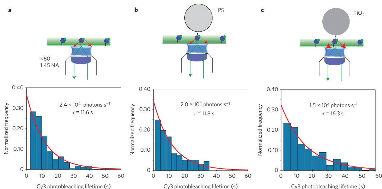
**Figure 3 | Cy3 photobleaching lifetimes increase in the presence of  $\text{TiO}_2$  colloids.** **a**, In the absence of colloids and colloidal lensing, Cy3-labelled streptavidin had a mean lifetime of 11.6 s under TIR excitation with a  $\times 60$  1.45 NA objective (excitation intensity 3.3 mW). **b**, The mean photobleaching lifetime with polystyrene colloids (PS) stayed nearly the same at 11.8 s. **c**, In the presence of  $\text{TiO}_2$  colloids, the lifetime increased to 16.3 s.
